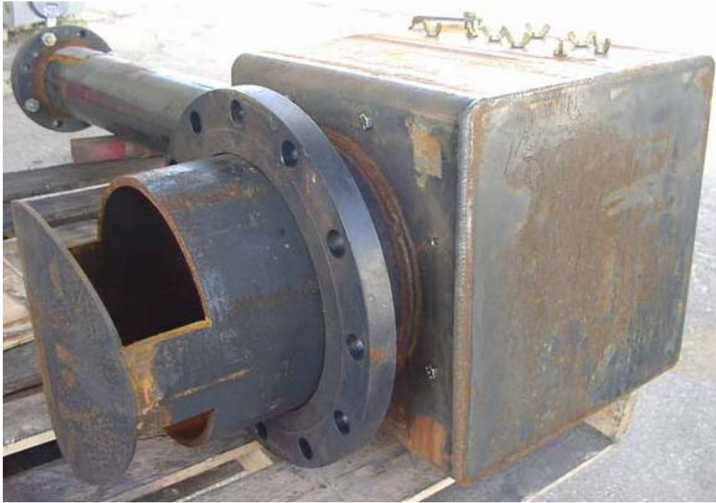
Figure 1. Client's Flameout FTPS Type B Foam Maker and Foam Chamber (Front View).
